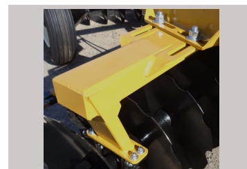
"W" Series with heavy 4" x 6" tubing and bearing hangers
