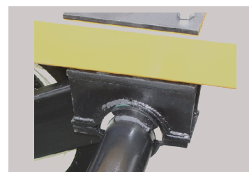
Replaceable nylon bearings on wheel mounts
